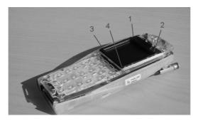
Snap the display assembly into the D-cover in the order shown.
