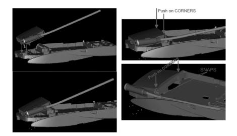
If antenna is being replaced, place a new antenna into the slot and press down (see arrows in above photos) to snap the assembly into place.
