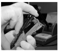
Mount the A-cover by fitting the guide fins into the D-cover first.
